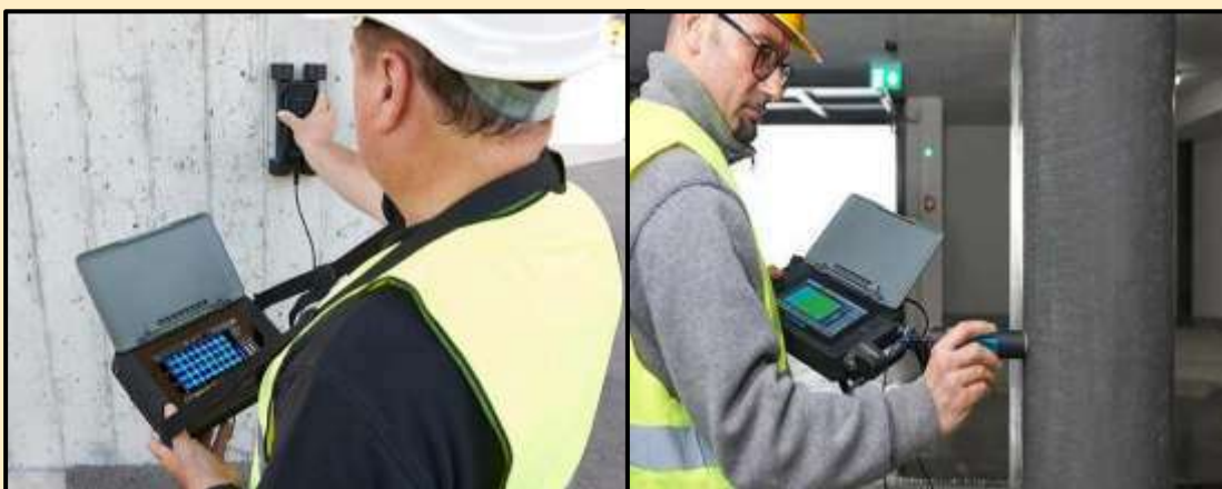
Figure 14: Profometer Test for Rebar Assessment and Corrosion Analysis
