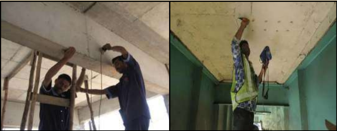
Figure 13: Ultrasonic Pulse Velocity Test on Beams and Slabs
