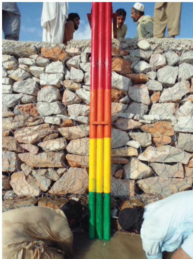
Early Warning System (EWS) monitoring water levels. Photo AHD
