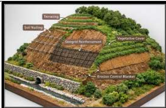
Geogrid Reinforced Retaining Wall
