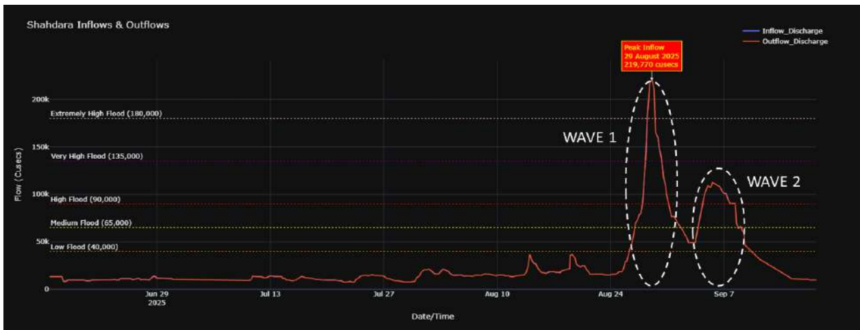
Figure: River Ravi flood waves 1 & 2 at Shahdara, Lahore
