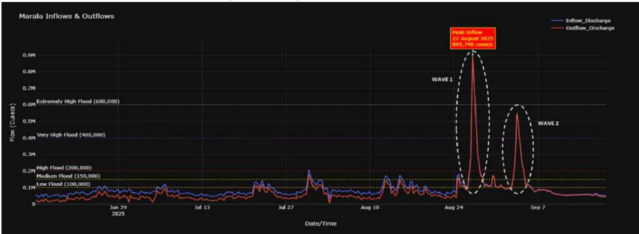
Figure: Flood waves 1 & 2 at Marala Headworks
